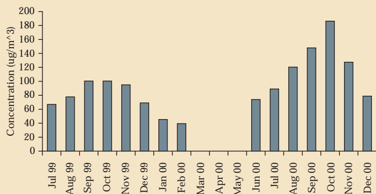
Figure 8.2: A record of near-ground ozone concentrations at Maun, in the north of Botswana (Botswana Department of Mines). Maun is far from any industrial pollution source, but close to the main centre of wildfire emissions.
