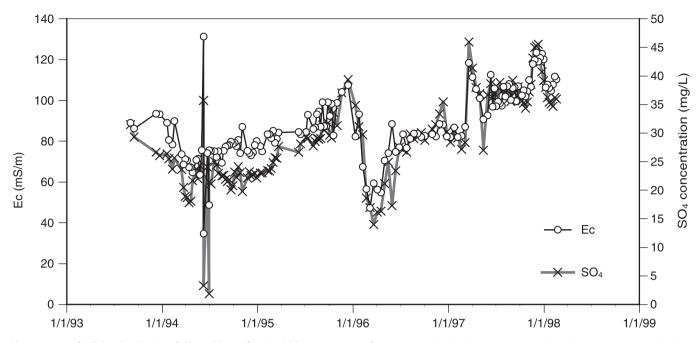
Figure 15.7. Salinization in the Olifant River, South Africa, 1993–98. Changes in electrical conductivity and sulphates measured in the Olifant River showing decreasing quality, attributed largely to coal mining activities. The Ec is a measure of the salt in the water. (S. African Dept. of Water Affairs and Forestry 1999 gauging station B3H017Q01)
